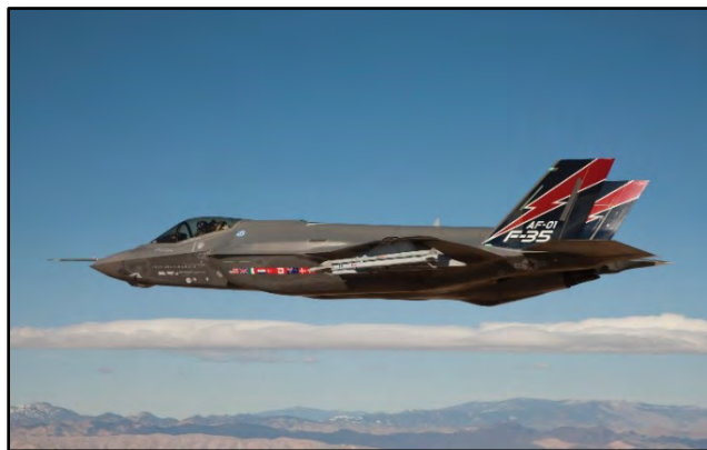
The F-35A combines internal weapon bays and expanded fuel capacity to permit low visibility penetration of enemy air defenses.
