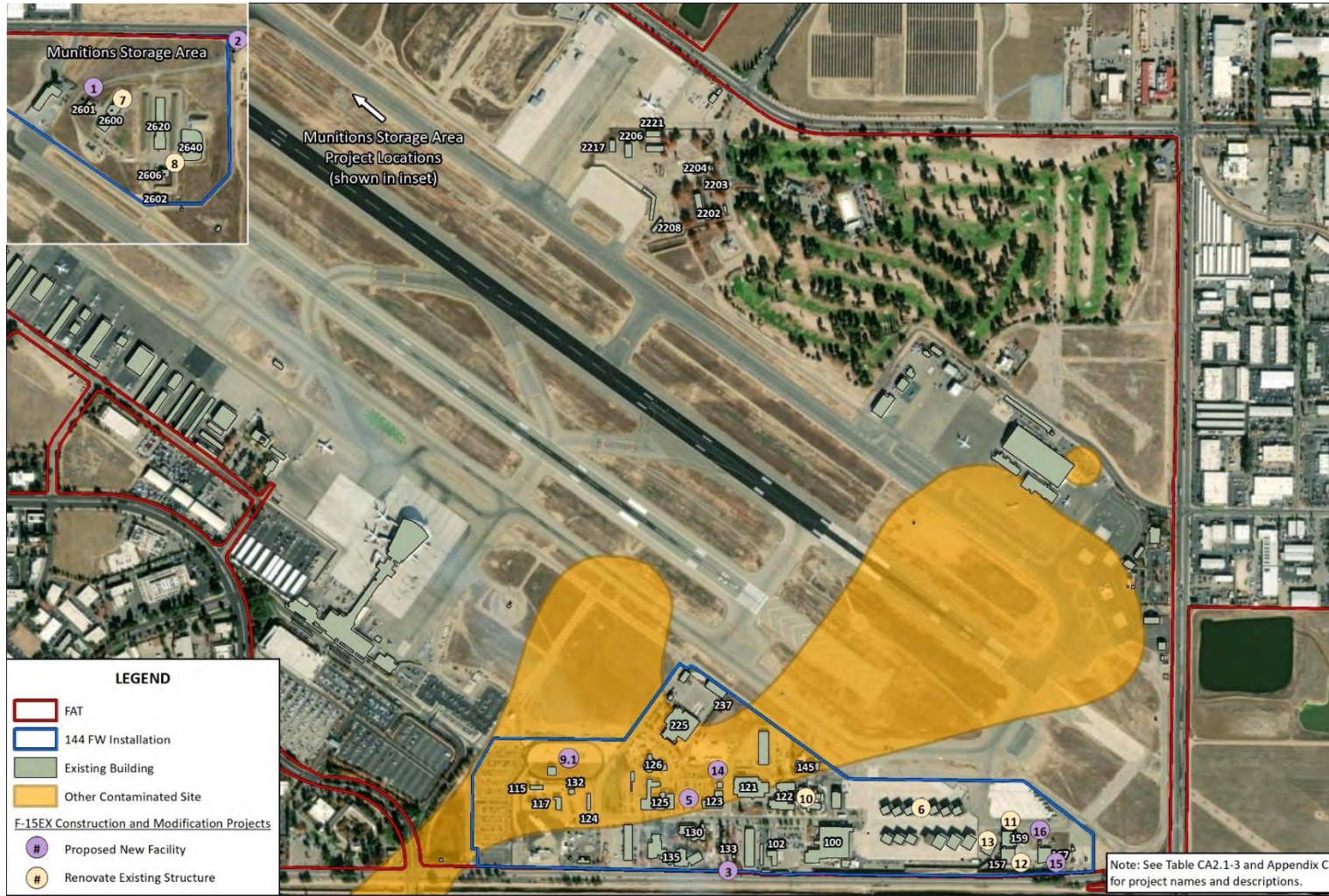
Figure CA3.11-3 IRP Sites and OHF Area 1 TCE Plume within the Vicinity of the Proposed Construction for the F-15EX at Locational Scenario 1 at the 144 FW Installation at Fresno Yosemite International Airport (FAT)
