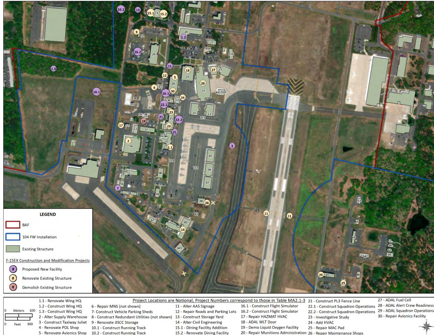
Figure MA2.1-1 Proposed Construction and Modifications for the F-15EX Beddown at the 104 FW at Westfield-Barnes Regional Airport (BAF)
