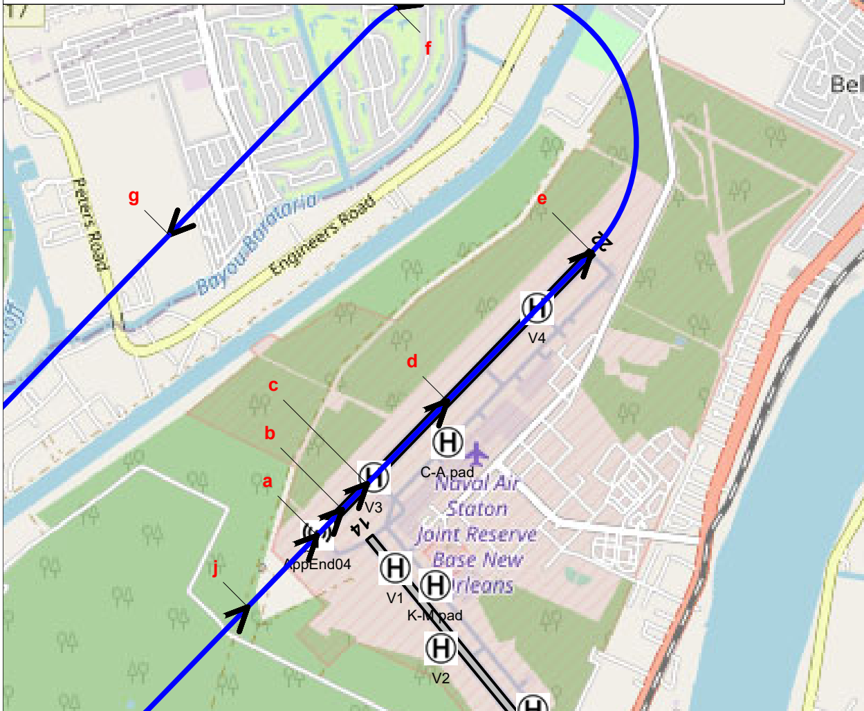
F-35A - Flight Profile F35_04C01 On Runway 4 - Runway 4, Flight Track F35_04C01 Closed VFR pattern in 04 direction
